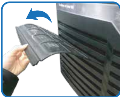
Remove air filter by sliding forward
